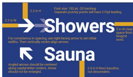
Example 2 in more detail: Clear space and set up. Yellow bars represent simplified distance measurements.
