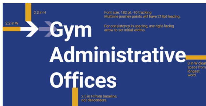
Example 1 in more detail: Clear space and set up. Yellow bars represent simplified distance measurements.
